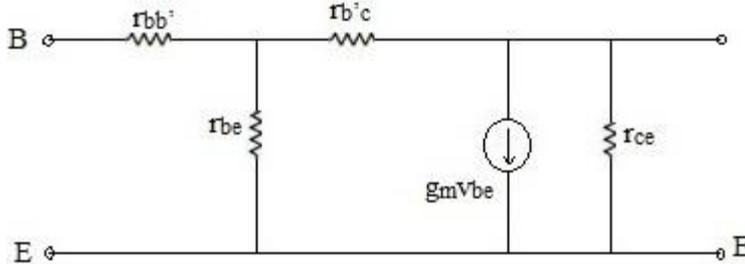
The High frequency model parameters of a BJT in terms of low frequency hybrid parameters is given below
