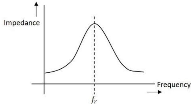
Impedance of the circuit decreases for the values above and below the resonant frequency  $f_r$ . Hence the selection of a particular frequency and rejection of other frequencies is possible.
