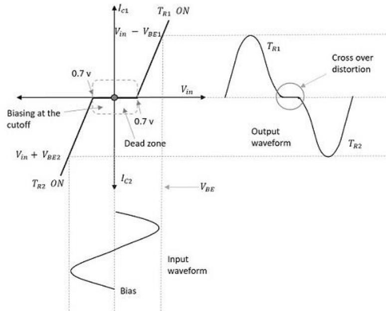
It is understood that this cross-over distortion is less pronounced for large input signals, where as it causes severe disturbance for small input signals. This cross over distortion can be eliminated if the conduction of the amplifier is more than one half cycle, so that both the transistors won't be OFF at the same time.
