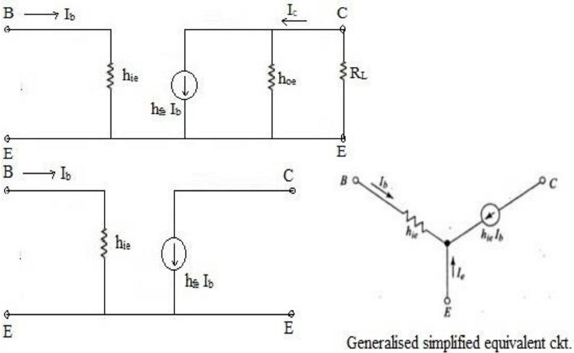
**Analysis of Common Emitter (CE) amplifier using simplified equivalent ckt**
