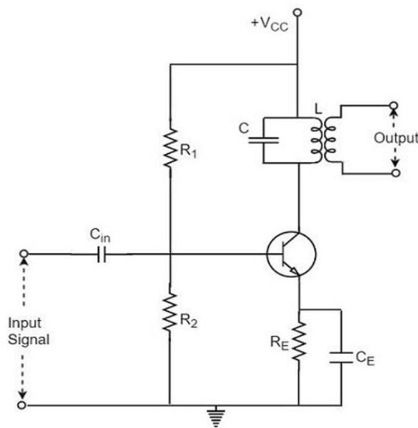
The tuner circuit is nothing but a LC circuit which is also called as **resonant** or **tank circuit**. It selects the frequency. A tuned circuit is capable of amplifying a signal over a narrow band of frequencies that are centered at resonant frequency.
