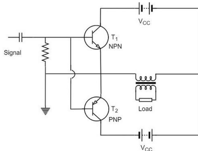
The above circuit employs a NPN transistor and a PNP transistor connected in push pull configuration. When the input signal is applied, during the positive half cycle of the input signal, the NPN transistor conducts and the PNP transistor cuts off. During the negative half cycle, the NPN transistor cuts off and the PNP transistor conducts.
