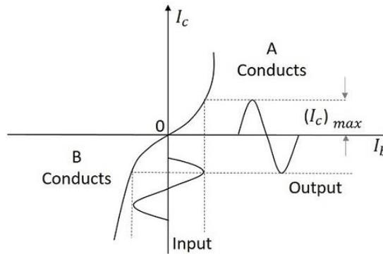
For the next half cycle, the transistor  $T_1$  gets into cut off condition and the transistor  $T_2$  gets into conduction, to contribute the output. Hence for both the cycles, each transistor conducts alternately. The output transformer  $T_{r3}$  serves to join the two currents producing an almost undistorted output waveform.
