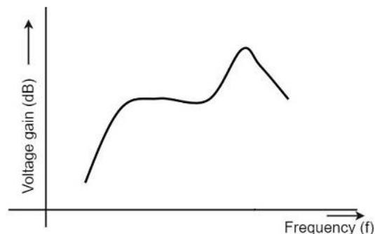
At low frequencies, the reactance of primary begins to fall, resulting in decreased gain. At high frequencies, the capacitance between turns of windings acts as a bypass condenser to reduce the output voltage and hence gain.
