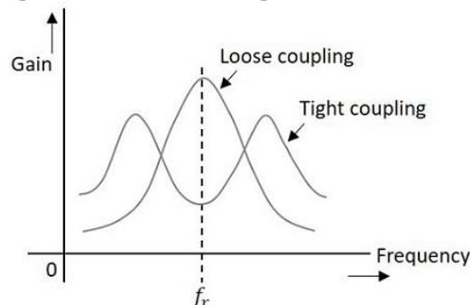
On the contrary, when the primary and secondary coils are brought close together, they have **Tight coupling**. Under such conditions, the reflected resistance will be large and the circuit Q is lower. Two positions of gain maxima, one above and the other below the resonant frequency are obtained.
