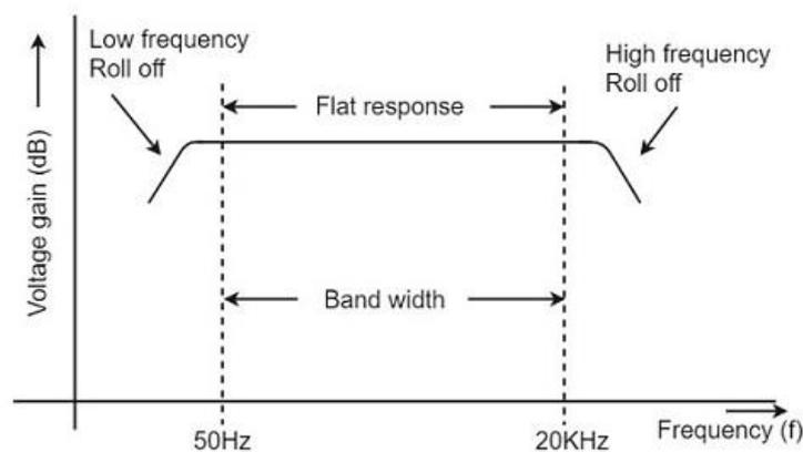
From the above graph, it is understood that the frequency rolls off or decreases for the frequencies below 50Hz and for the frequencies above 20 KHz. whereas the voltage gain for the range of frequencies between 50Hz and 20 KHz is constant.
