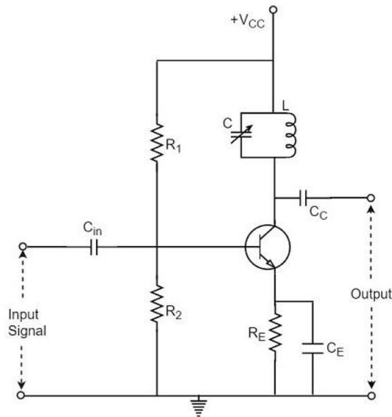
The output can be obtained from the coupling capacitor  $C_c$  as shown above or from a secondary winding placed at L.
