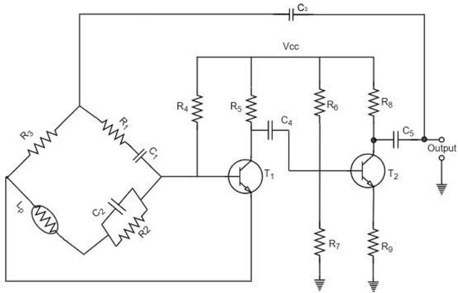
The transistor  $T_1$  serves as an oscillator and an amplifier while the other transistor  $T_2$  serves as an inverter. The inverter operation provides a phase shift of  $180^\circ$ . This circuit provides positive feedback through  $R_1C_1$ ,  $C_2R_2$  to the transistor  $T_1$  and negative feedback through the voltage divider to the input of transistor  $T_2$ .
