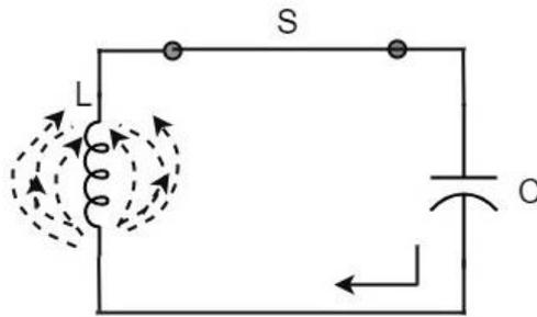
Now, let us move on to the next stage. Once the capacitor is discharged completely, the magnetic field begins to collapse and produces a counter EMF according to Lenz's law. The capacitor is now charged with positive charge on the upper plate and negative charge on the lower plate.
