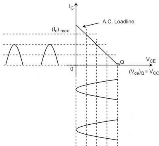
When the signal is applied, the circuit is forward biased for the positive half cycle of the input and hence the collector current flows. But during the negative half cycle of the input, the circuit is reverse biased and the collector current will be absent. Hence **only the positive half cycle** is amplified at the output.
