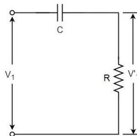
The output voltage  $V_1'$  across the resistor R leads the input voltage applied input  $V_1$  by some phase angle  $\phi^\circ$ . If R were reduced to zero,  $V_1'$  will lead the  $V_1$  by  $90^\circ$  i.e.,  $\phi^\circ = 90^\circ$ .
