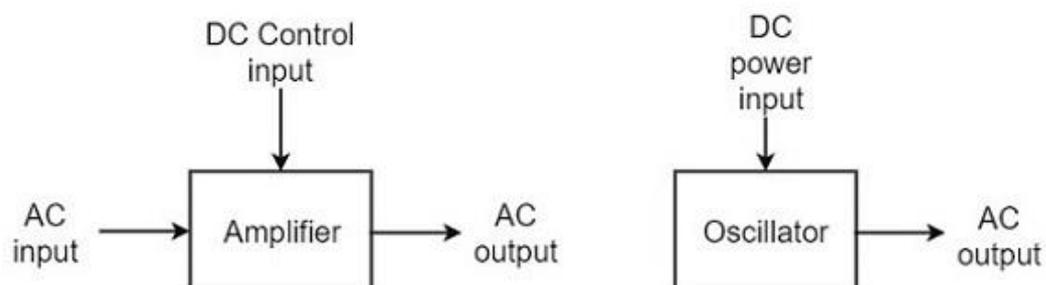
The frequency, waveform, and magnitude of a.c. power generated by an amplifier, is controlled by the a.c. signal voltage applied at the input, whereas those for an oscillator are controlled by the components in the circuit itself, which means no external controlling voltage is required.
