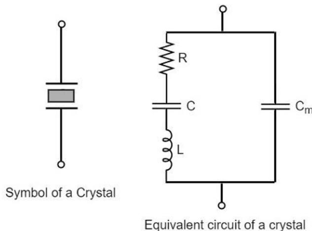
The above equivalent circuit consists of a series R-L-C circuit in parallel with a capacitance  $C_m$ . When the crystal mounted across the AC source is not vibrating, it is equivalent to the capacitance  $C_m$ . When the crystal vibrates, it acts like a tuned R-L-C circuit.
