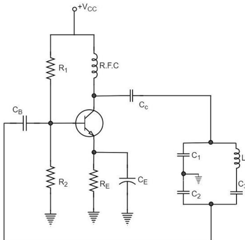
The operation of Clapp oscillator circuit is in the same way as that of Colpitts oscillator. The frequency of oscillator is given by the relation,
