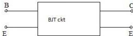
For small signal behaviour the transistor at its input port behaves as a resistor.
