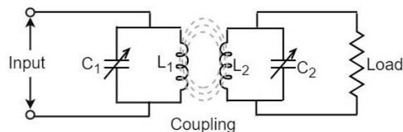
When the coils are spaced apart, the flux linkages of primary coil  $L_1$  will not link the secondary coil  $L_2$ . At this condition, the coils are said to have **Loose coupling**. The resistance reflected from the secondary coil at this condition is small and the resonance curve will be sharp and the circuit Q is high as shown in the figure below.
