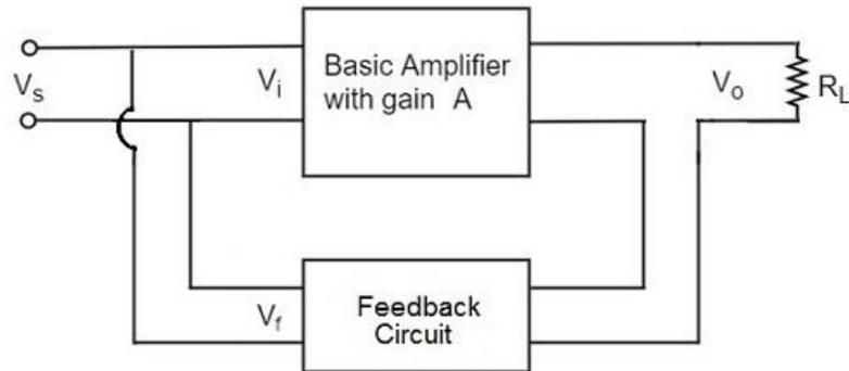
As the feedback circuit is connected in series with the output, the output impedance is increased and due to the parallel connection with the input, the input impedance is decreased.
