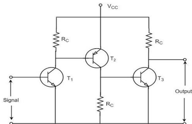
The transistor in the first stage will be an NPN transistor, while the transistor in the next stage will be a PNP transistor and so on. This is because; the variations in one transistor tend to cancel the variations in the other. The rise in the collector current and the variation in  $\beta$  of one transistor gets cancelled by the decrease in the other.
