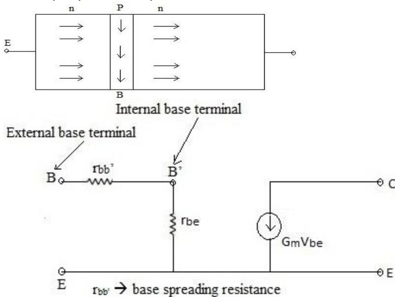
Because the base (B) is lightly doped all the depletion region lies entirely in the Base region. So, when the collector.
