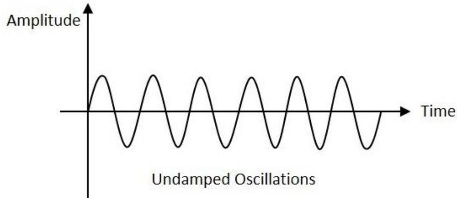
Undamped oscillations are generally produced by the oscillatory circuits that produce no power losses and follow compensation techniques if any power losses occur.
