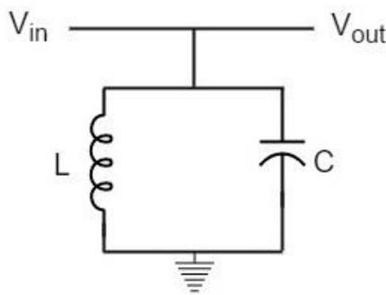
At resonant frequency, a parallel resonant circuit offers high impedance which does not allow high current through it. A parallel resonant circuit offers increasingly low impedance to the frequencies far from the resonant frequency.
