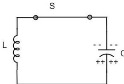
Once the capacitor is fully charged, it starts to discharge to build up a magnetic field around the coil, as shown in the following circuit diagram.
