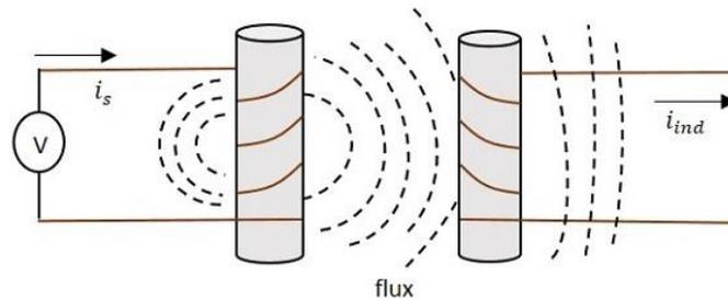
The current  $i_s$  in the figure indicates the source current while  $i_{ind}$  indicates the induced current. The flux represents the magnetic flux created around the coil. This spreads to the secondary coil also. With the application of voltage, the current  $i_s$  flows and flux gets created. When the current varies the flux gets varied, producing  $i_{ind}$  in the secondary coil, due to the Mutual inductance property.
