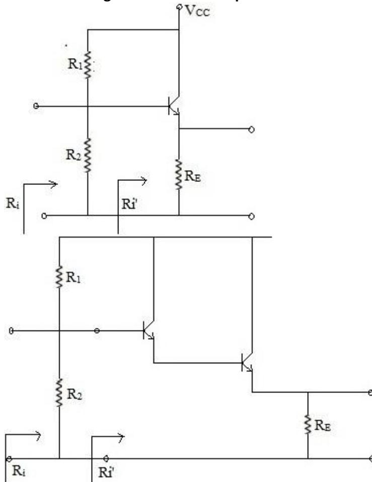
Effective input resistance  $R_i = R_1 \parallel R_2 \parallel R_i'$  where  $R_i'$  is a large input resistance of emitter follower or Darlington ckt.
