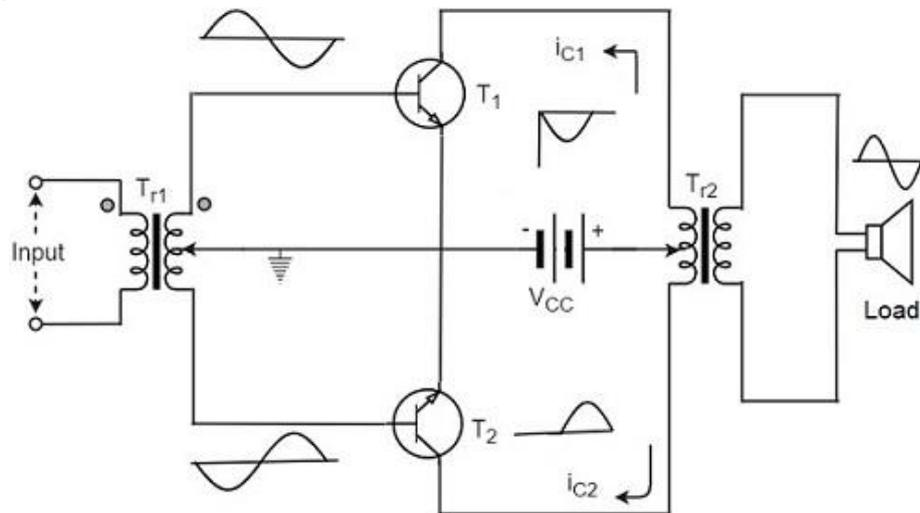
The circuit operation of class B push pull amplifier is detailed below.
