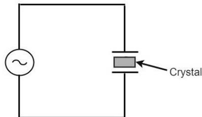
If an AC voltage is applied, the crystal starts vibrating at the frequency of the applied voltage. However, if the frequency of the applied voltage is made equal to the natural frequency of the crystal, **resonance** takes place and crystal vibrations reach a maximum value. This natural frequency is almost constant.
